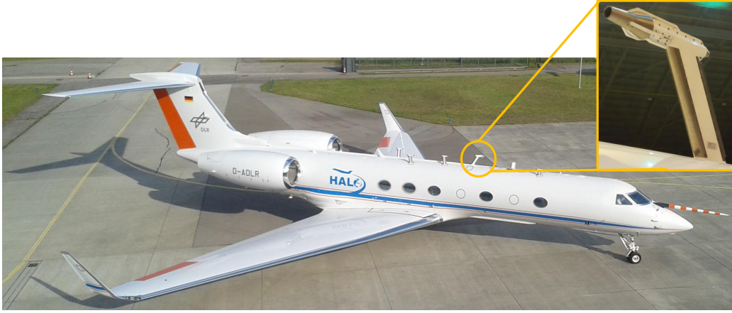
Figure 4: Picture of the German research aircraft HALO and the aerosol inlet HASI mounted on top of the fuselage.
