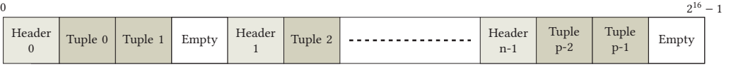
(b) BD-Tree and HLN-Tree leaf node design. The number of tuples in each subnode is limited to 3 instead of 255 in this sketch to keep the figure small.
