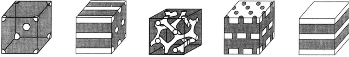
Figure 2.3: Schematic representation of diblock copolymer mesophases: spheres (S), cylinders (C), gyroid (G), perforated lamellae (PL), lamellae (L) (from left to right).
