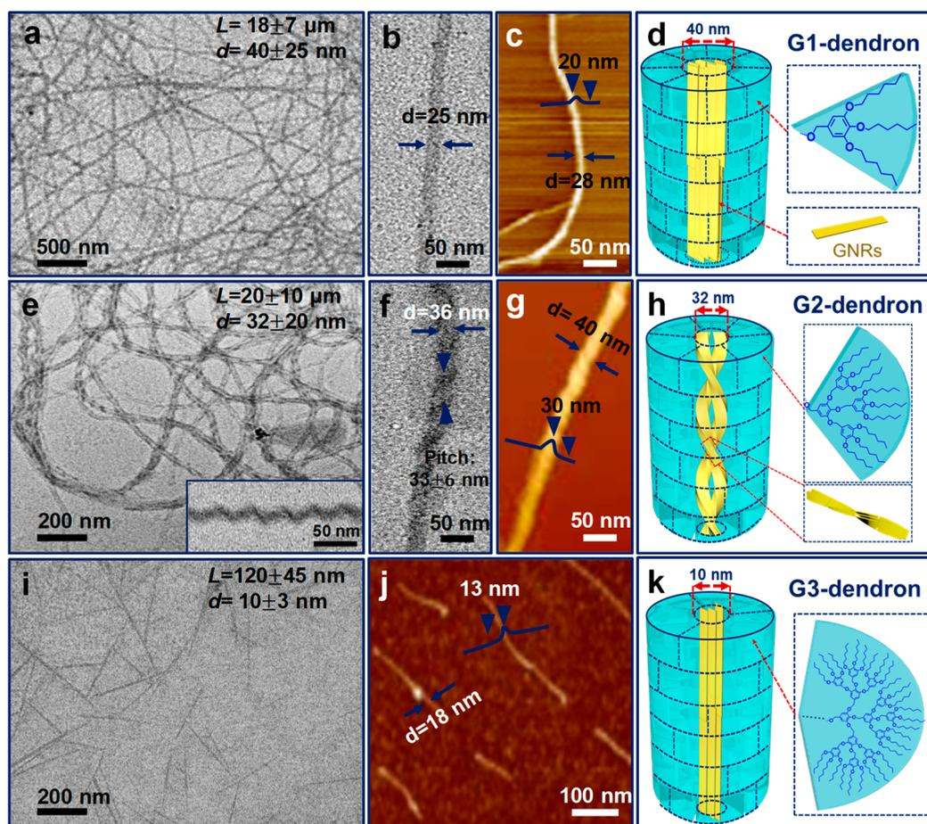
**Figure 3.** TEM images, AFM height profiles, and the proposed aggregation models of the GNR superstructures in THF. (a–d) GNR-G1 nanowires; (e–h) GNR-G2 helices (inset in panel e shows a typical cryo-TEM image); (i–k) GNR-G3 nanofibers. In the schematic aggregation models, the short alkyl chains between the GNR backbones and dendrons are omitted; the near-fan architected dendrons are presented as “regular fans” separated by dashed lines, which are not the actual “borders” among the dendrons.
