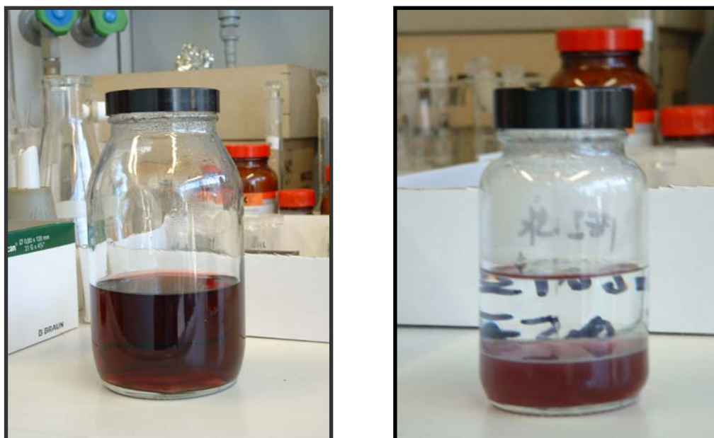
Figure 7-13. Photos of gold nanoparticle solutions with 12nm particles (left) and transported by the HPEI10K-C16 0.6 N + 0.4 capsules (right) into the chloroform phase
