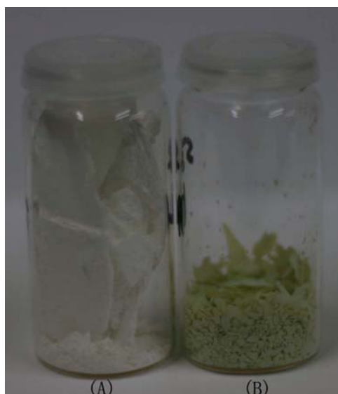
Figure 5-8. PMMA polymers after purification by precipitation in methanol (A) with HPEI25K-EA 0.79 as macroligand; (B) with PMDETA as ligand
