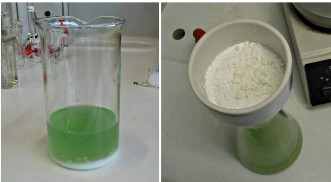
Figure 5-7. Separation of the complex of HPEI25K-EA 0.79 /CuCl from the polymerization mixture. Left: after precipitation; Right: after filtration.
