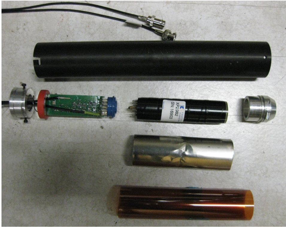
Figure 42: The soft iron shielding, the voltage divider, the PMT, the \mu metal shielding and the capton insulation of H1. The aluminium part serve as a fixation.
