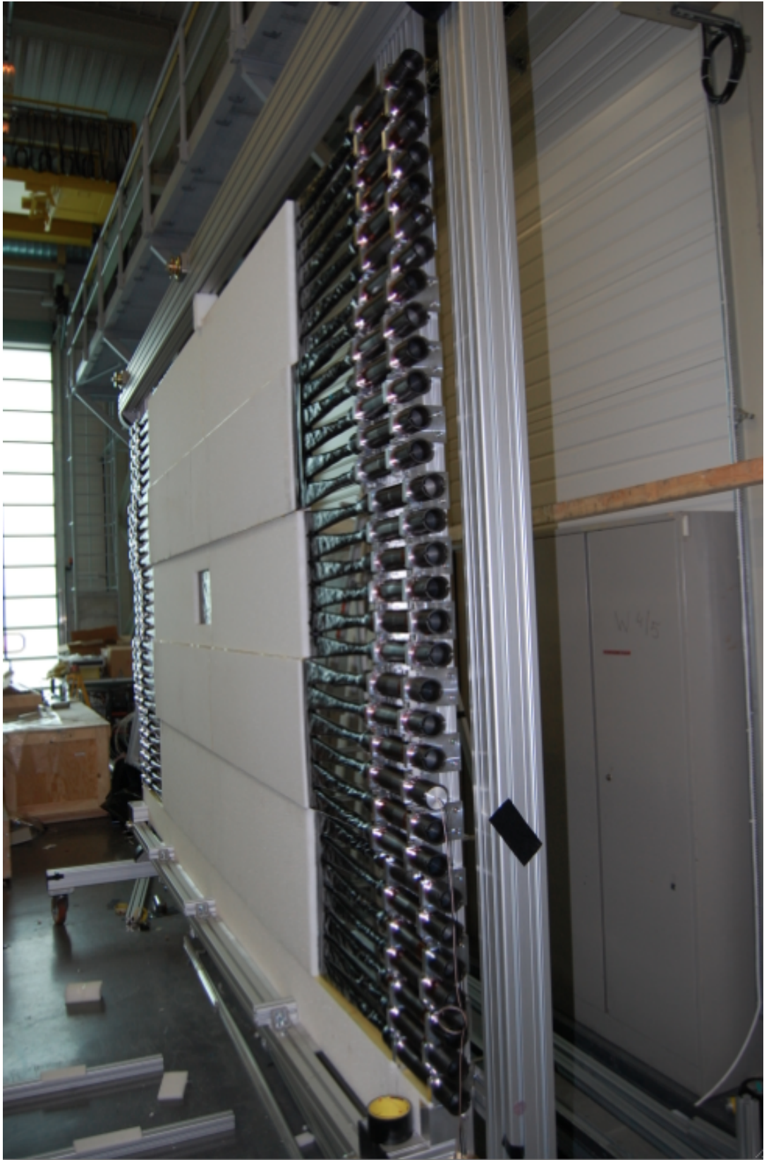
Figure 122: Picture of H1 during construction, attached to the mounting frame with wheels.
