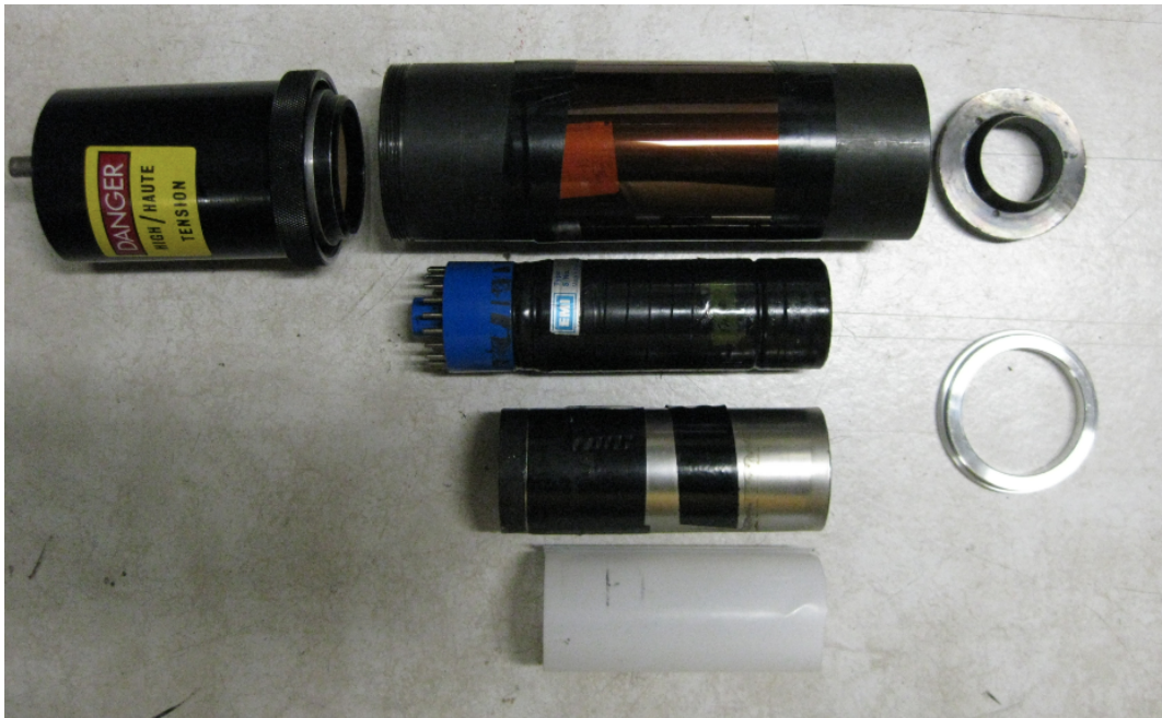
Figure 44: The PMT, the \mu metal shielding, the soft iron shielding, the Teflon insulation, the metal connector and the voltage divider used in H2.
