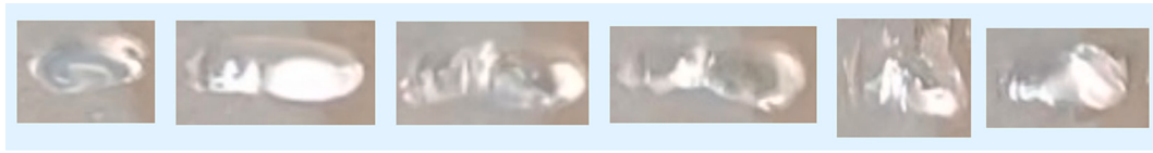
Fig. 2. Time sequence of drop floating in laminar air stream with extreme oscillations in horizontal mode. \Delta t = 0.05 s. From video recording with a mobile phone.
