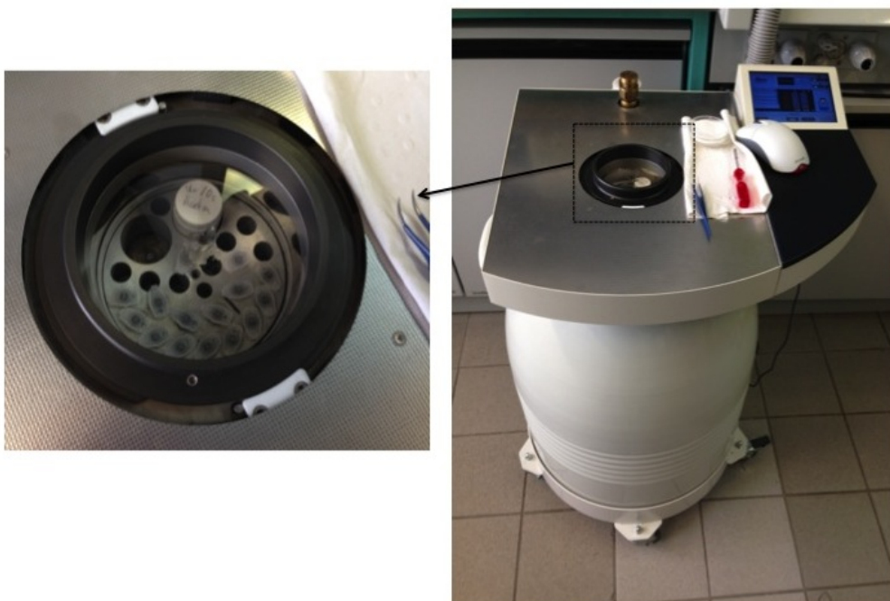
Figure 9.3. EM AFS Freeze substitution machine. Enlargement view of the loading stage.
