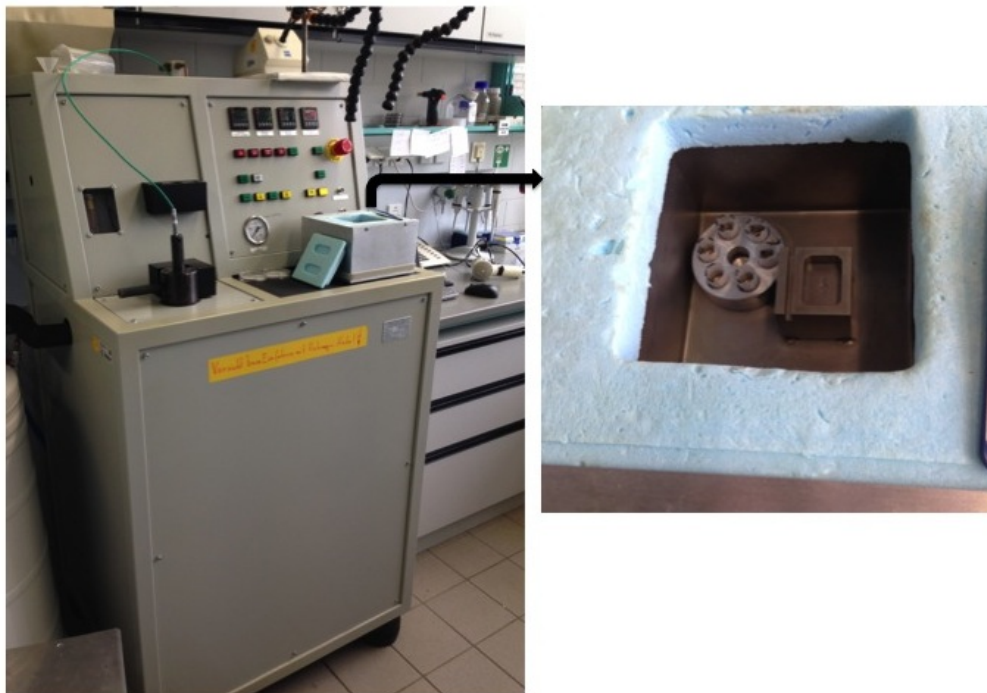
Figure 9.2. High Pressure Freezing Machine. Enlargement view of the aluminium box for storage of grids.
