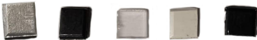
Fig. 3.2.3 The materials examined on the effect of biofilm formation. The different types of materials were cut to a square shape and analyzed for their impact on biofilm formation. From left to right: S235 steel, PE, PETG, PC, and PS.
