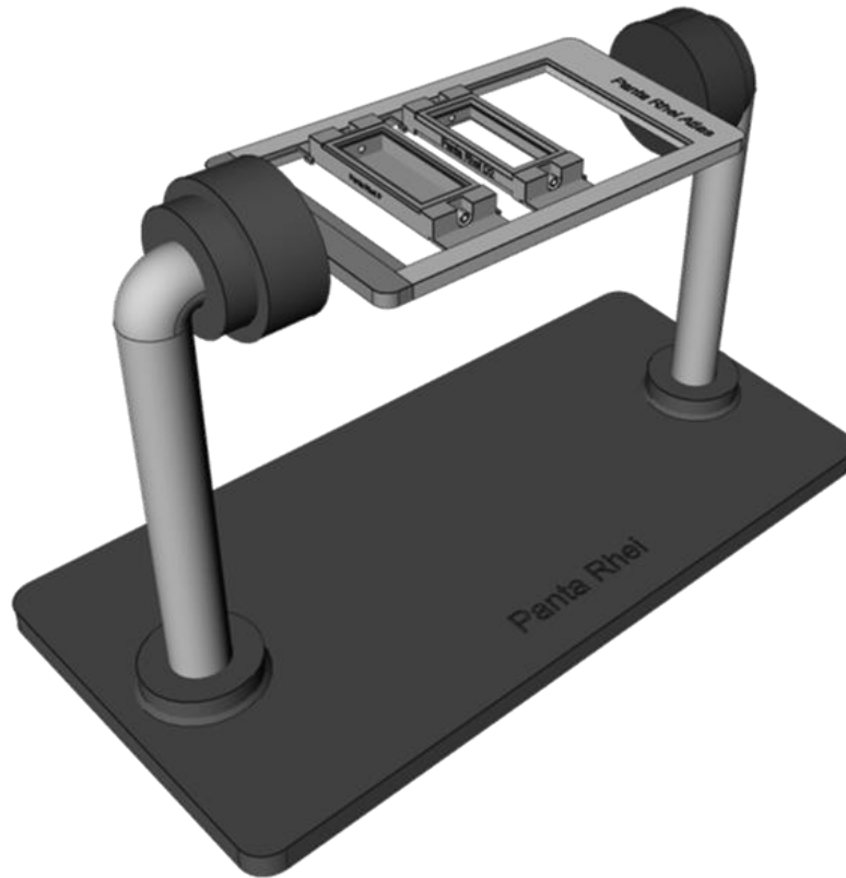
Fig. 3.1.9 The redesigned Pantia Rhei Atlas carrying Pantia Rhei flow cells. The Pantia Rhei Atlas was supplied with a special groove to accommodate one or more Pantia Rhei flow cells. With the help of the swivel joints on the sides, control by a stepper motor is enabled. An operation in combination with a frame joint was not necessary for the angular settings.
