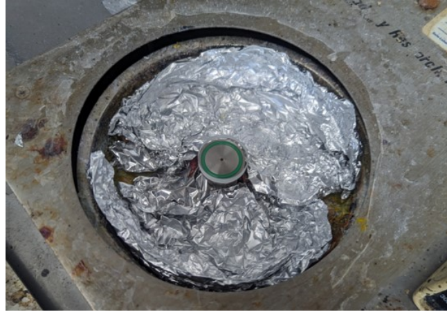
FIGURE 3.9: One of the UV windows for the n2EDM precession chamber mounted in the spin coater to coat them with dPE to increase the Fermi pseudo-potential.
