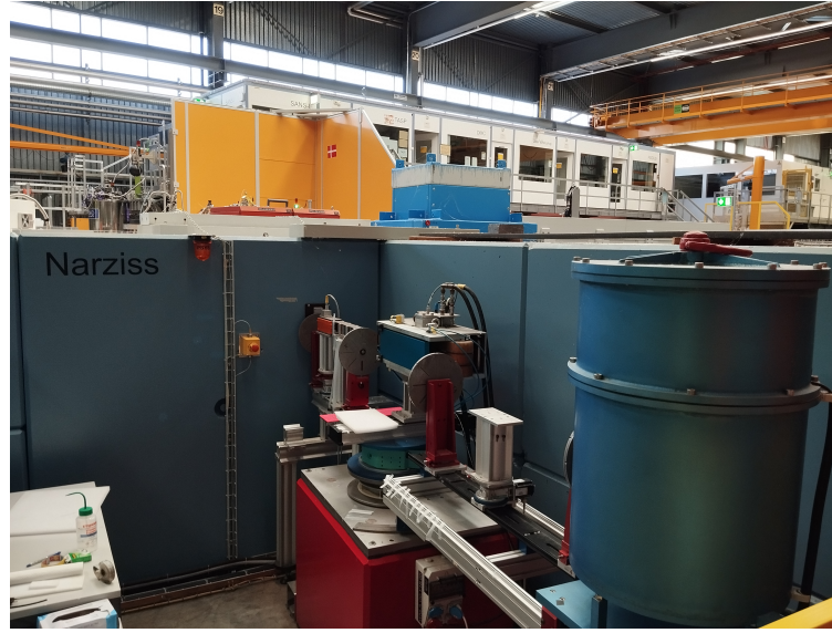
FIGURE 3.6: The cold neutron beam line NARZISS which was used to measure the Fermi pseudo-potential of the coating of the insulating rings for the n2EDM experiment.
