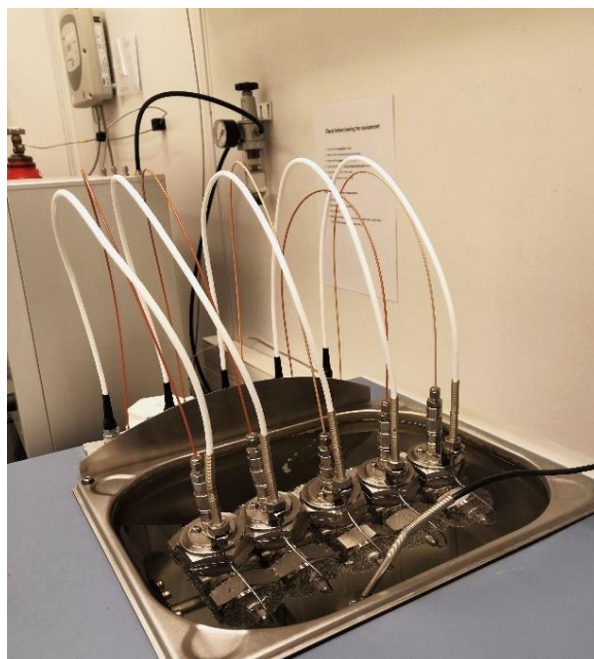
Figure 4: High-pressure rocking cells for testing KHI performance.
