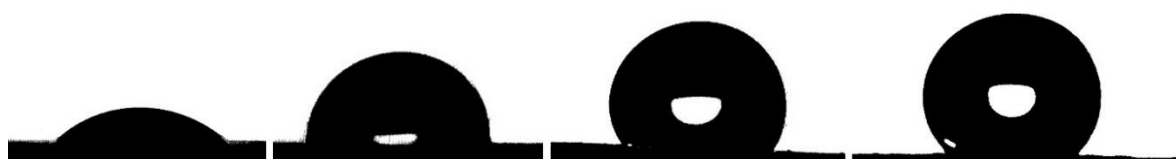
Figure 9: Water drops on uncoated and coated surfaces. From left to right: uncoated glass ( 42^\circ ), C8 coated glass ( 96^\circ ), C8 coated cellulose ( 115^\circ ), uncoated Teflon ( 128^\circ ).
