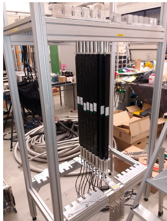
Fig. 2. Image of a first wall module installed in the support frame during assembly.
