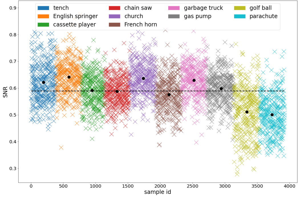
Fig. 5.2.: signal to noise ratio (SNR) of Imagenette classes. The values are produced using ResNet18. Each colored dot corresponds to a single sample. The dotted line describes the overall average SNR.
