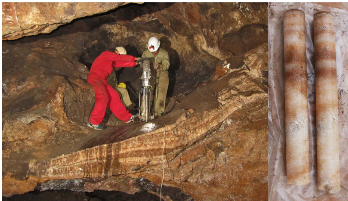
Figure 3.2: (Left panel) Sampling of the Cueva Victoria flowstone sequence using a mobile drilling machine (picture courtesy of C. Rossi). (Right panel) The obtained cores have a length of ca. 50 cm and a width of 5 cm.
