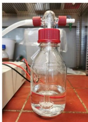
Figure S39: Washing bottle with 200 mL of 1 mol·L -1 NaOH.
