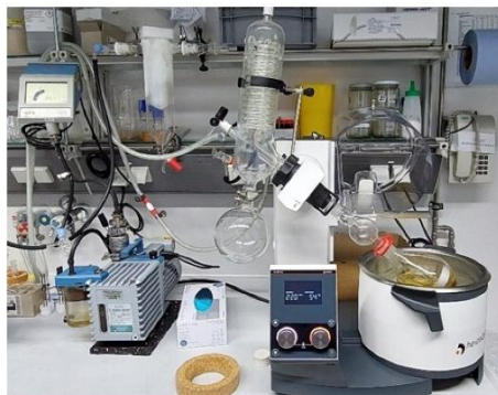
Figure S3.63: Distillation system for the distillation of 1,2-dichloroethyl acetate ( 8 ).
