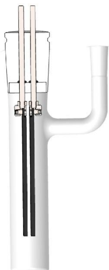
Figure S1.8: Cross-section of a NS34 Teflon lid for two (120 x 23 x 3) mm electrodes.
