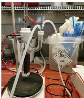
Figure S38: Electrolysis cell with connected electrodes and nitrogen gassing.
