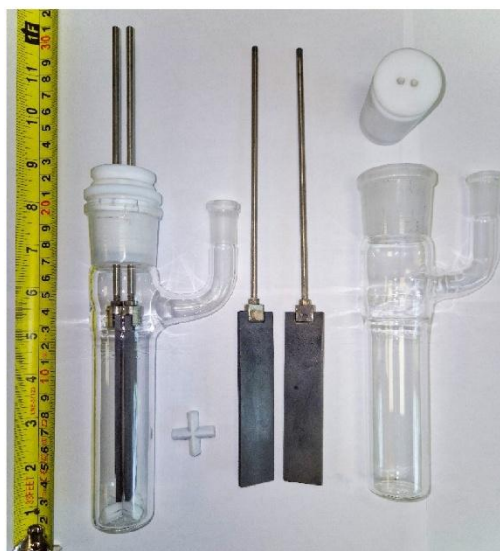
Figure S1.11: 50 mL glass vial with (120 x 23 x 3) mm isostatic graphite electrodes.
