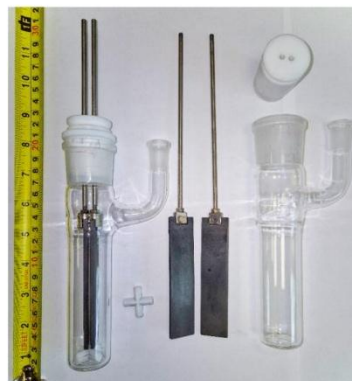
Figure S6: 50 mL glass vial with (120 x 23 x 5) mm isostatic graphite electrodes attached to titanium holders.
