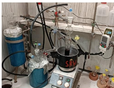
Figure S3.65: Distillation system for the distillation of 2,3-dichloro-1-propanol ( 10 ).
