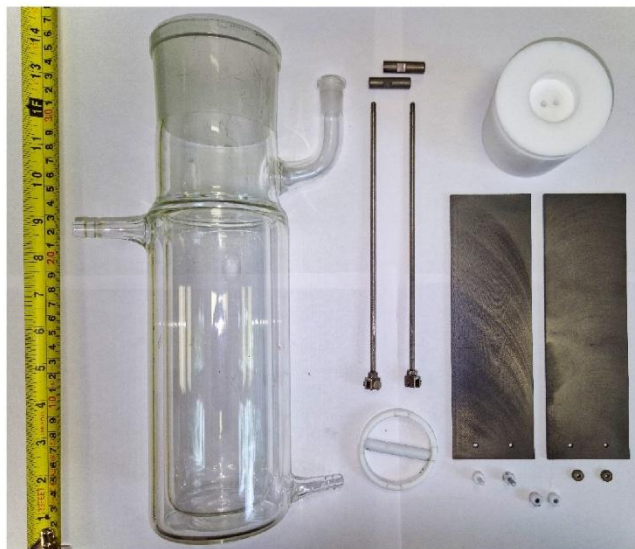
Figure S1.13: 500 mL glass vial with (225 x 58 x 3) mm isostatic graphite electrodes.
