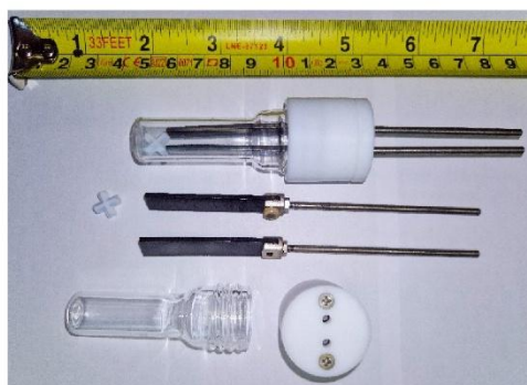
Figure S1.2: 5 mL glass vial with a stirring bar, various lids for different electrode types and isostatic graphite electrodes attached to titanium contacts.
