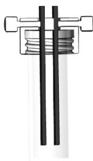
Figure S1.7: Cross-section of a Teflon lid for two (70 x 10 x 2) mm electrodes.
