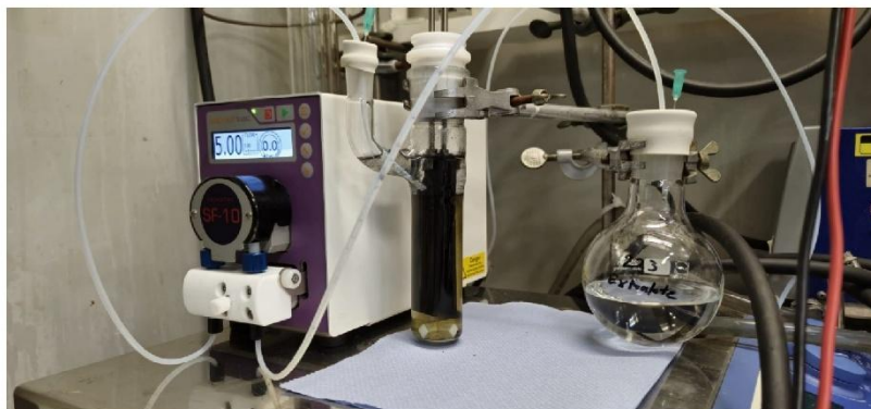
Figure S3.61: Extraction of methyl 10-undecenoate (3) and methyl 10,11-dichloroundecanoate (4) with heptane after electrolysis.
