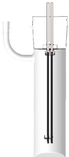
Figure S1.12: Cross-section of a NS71 Teflon lid for two (225 x 58 x 3) mm electrodes.
