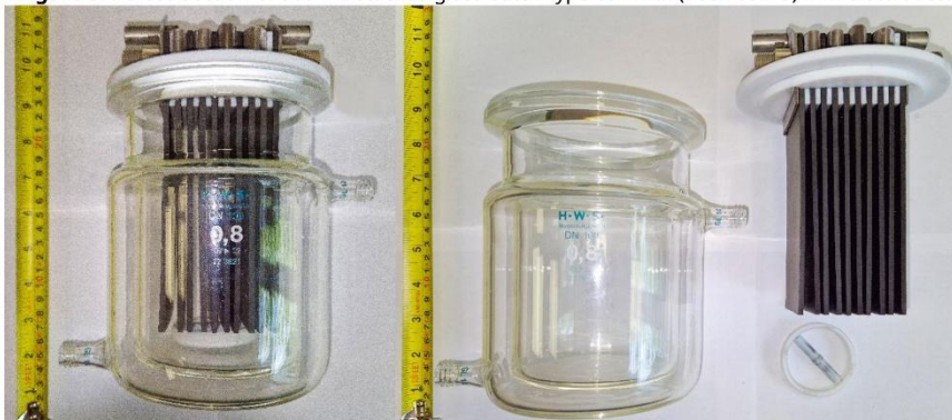
Figure S8: 500 mL stacked glass batch-type cell with (160x 65 x 3) mm isostatic graphite electrodes.
