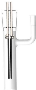
Figure S5: Cross-section of an NS34 Teflon lid for two (120x 23 x 3) mm electrodes.
