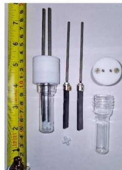
Figure S2: 5 mL glass vial with a stirring bar, Teflon lid and isostatic graphite electrodes attached to titanium holders.
