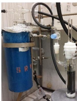
Figure S40: Electrolysis cell with connected cooling trap.
