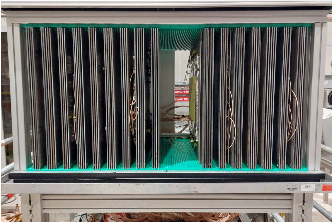
(a) Picture of the open ECAL layer stack at the SPS TB showing the slot structure and layer ordering.
