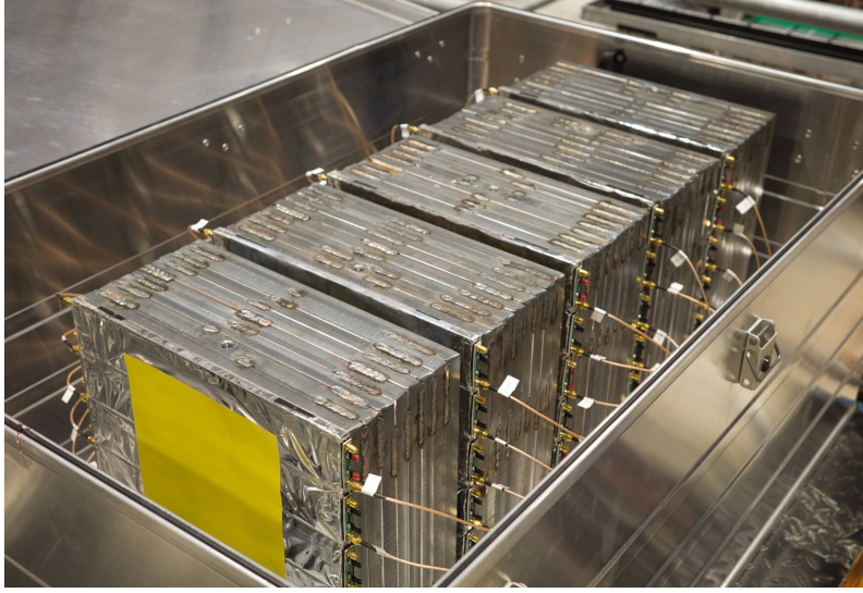
Figure 49: Picture of the HCAL prototype at the SPS TB. The ECAL and beam pipe are in the top right direction.
