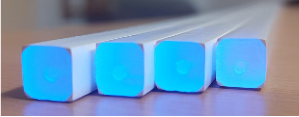
Figure 42: Picture of the 1 \times 1 \times 20 \text{ cm}^3 coextruded scintillators from Fermilab under UV light with the \text{TiO}_2 coating on the outside and the fiber channel in the center.
