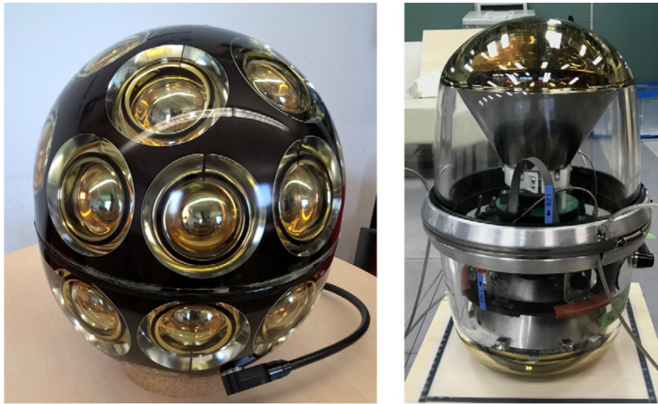
Figure 8.2: Prototype of the mDOM (left) and the D-Egg (right). Both types of modules will be used to instrument the seven Upgrade strings. Figure taken from Ref. [43].
