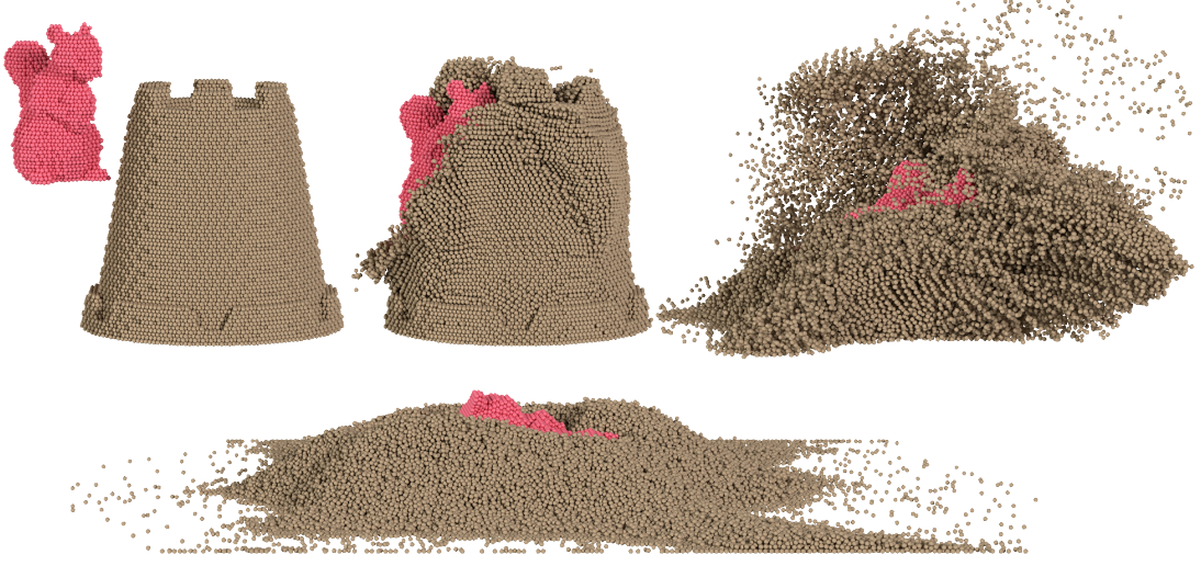
Figure 4.3: A rigid body (squirrel), represented by a collection of particles, is thrown into a tower of granular particles. The interaction between the granular particles and the rigid body particles is simulated, with the rigid body particles being constrained to maintain the shape of the squirrel through a shape-matching constraint. This results in a two-way coupling between the granular material and the rigid body.
