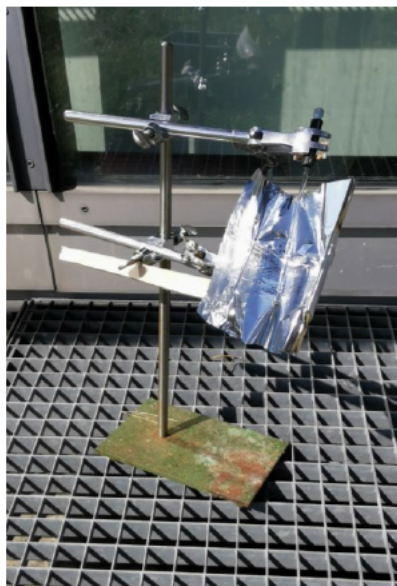
Figure 30: Set-up for solar irradiation. An NMR tube is held by a clamp and a reflector made from half-circular plastic tube and a silver-coated foil is used for focussing solar light.
