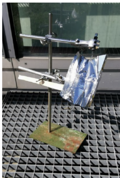
Figure 7: Set-up for solar irradiation. An NMR tube is held by a clamp and a reflector made from half-circular plastic tube and a silver-coated foil is used for focussing solar light.
