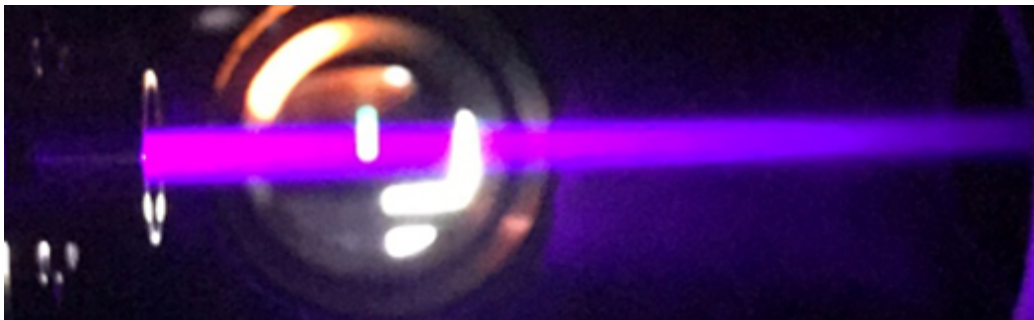
Figure 5: Picture of fluorescence-light of ^{164}\text{Dy} in the gas jet of JetRIS at 404.5 nm.
