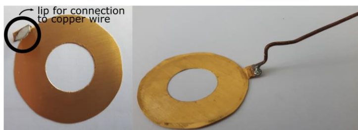
Figure 2-4: Image of the gold foil ring used to connect to the graphene layer and the finished gold foil ring including the attached copper wire.
