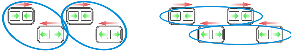
Figure 71: Illustration on how the fake configurations (right) are formed compared to the consecutive ones (left). The green arrows correspond to the polarisation direction of the target cells and the red ones show the direction of the solenoid field. The blue circles illustrate how the groups are formed.
