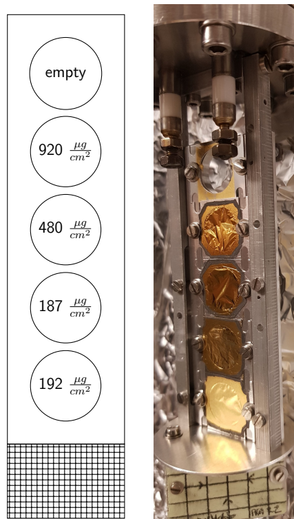
Figure 3.11.: Sketch of the target holder on the left. The numbers inside the circles give the thickness of the gold, and the positions as in table 3.1 are from bottom to top. Photograph of the target holder on the right with the gold foils. The ladder measures 130 mm in length.
