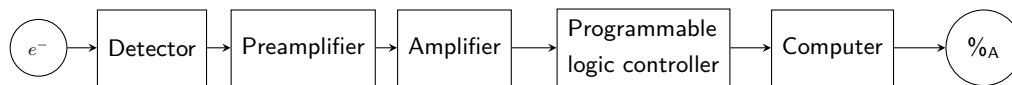
Figure 4.2.: Scheme of the signal processing from electron to asymmetry. If an electron hits the detector, the signal gets pre-amplified and fed into an amplifier. This analog signal is fed into a programmable logic controller, which is transferred into the computer. This signal is then used for the data analysis and the asymmetry in its unit % A is calculated.
