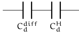
Figure 4: Schematic of the Stern model in Figure 3c, depicting the double layer as two capacitors in series.
