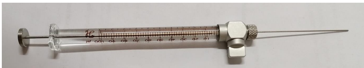
Figure S10: A 100 µL Hamilton™ Gastight™ SampleLock™ twist-valve syringe used to take samples for gas chromatography.
