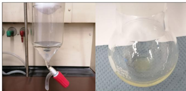
Figure 6. Left: Easy recovery of the HFIP/MeCN solvent mixture from the crude reaction medium using vacuum distillation/condensation into a cooling trap. Right: Isolated sulfonamide product of the reaction which used a SO 2 stock solution that was made from recovered HFIP/MeCN (see Supporting Information for more details).
