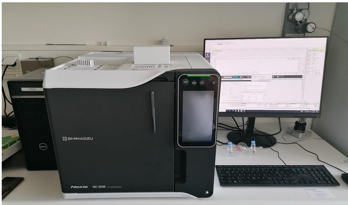
Figure S9: A Shimadzu Nexis GC-2030 with helium as carrier gas and a BID (barrier ionization discharge) detector used for analysis, kindly provided by Dr. Simon Clausing from the group of Prof. Dr. Carsten Streb, Mainz University.
