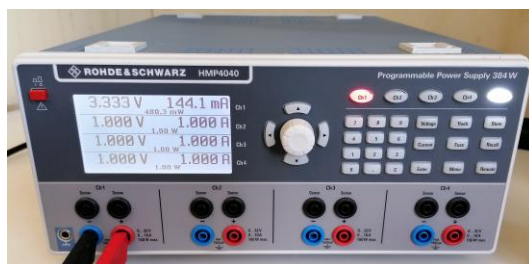
Figure 10. A commonly used power supply for galvanostatic electrolysis.
