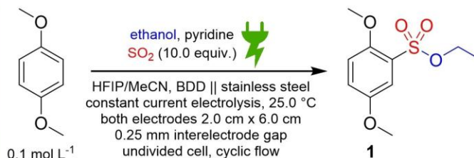
Scheme 1. Electrochemical multi-component synthesis of ethyl 2,5-dimethoxy-benzenesulfonate ( 1 ) directly from 1,4-dimethoxybenzene, \text{SO}_2 , and ethanol in an undivided flow electrolysis cell.
