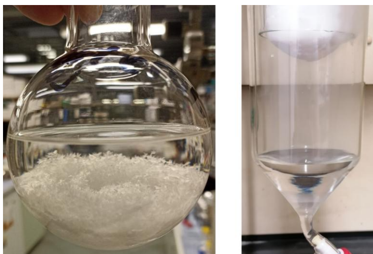
Figure 15. Recrystallization and distillation are simple and inexpensive purification techniques. Left: recrystallization of lanosterol from MeCN. Right: MeCN / HFIP / SO 2 in a cooling trap. [71]
