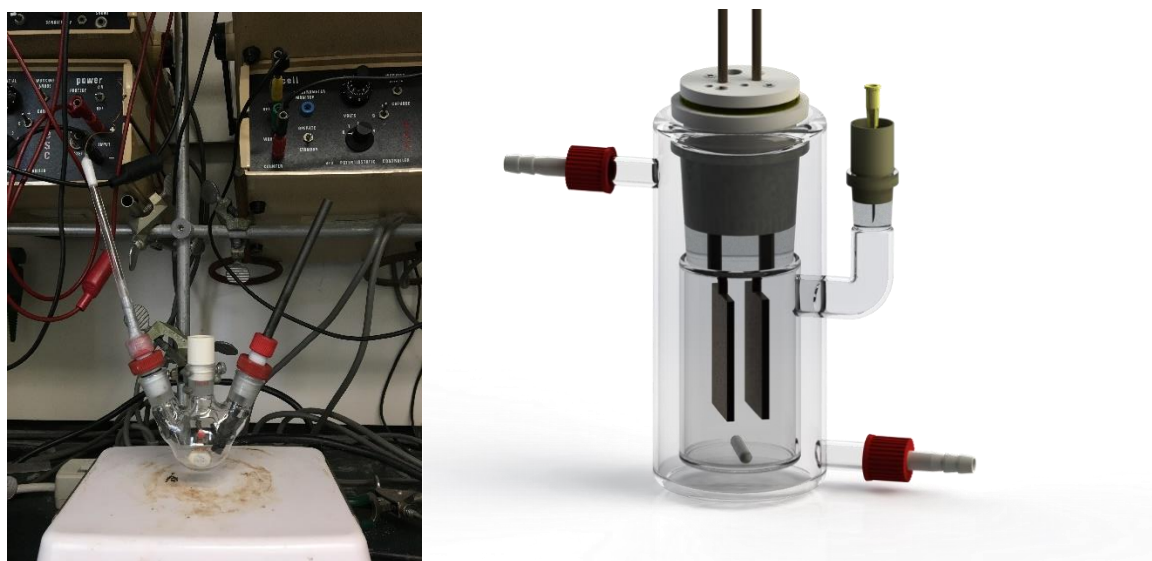
Figure 1: Electrochemical set-up in a three-necked flask (electrolysis protocol A) and the 25 mL beaker-type glass cell (electrolysis protocol B).
