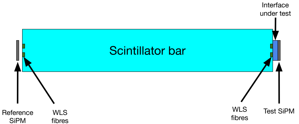
Figure 5.35: Visualisation of the setup. The left SiPM is set with a reference interface which remains unmodified throughout the study. The right SiPM is connected to a custom interface which changes during the study. For the measurement where the interface under test is a simple airgap, the reference SiPM yields an amplitude A_{\text{ref,Airgap\_ref}} whereas the test SiPM yields A_{\text{test,Airgap\_ref}} . When the interface under test is set to be “active”, the reference SiPM records A_{\text{ref,\_test}} whereas the test SiPM records A_{\text{test,\_test}} .
