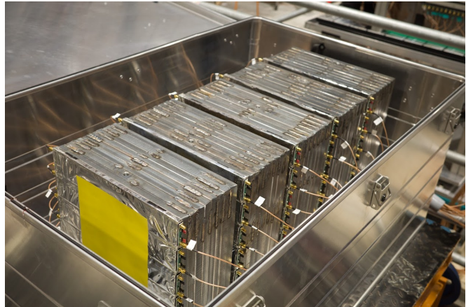
Figure 7.35: ECAL (left) and HCAL (right) prototype built and operated in TB4. The beam comes from the right.
