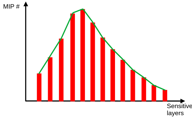
Figure 7.19: Principle of interpolation-based energy reconstruction: each red bar represents a sensitive layer with the green curve representing the interpolated longitudinal shower shape which is similar to the total shower energy.
