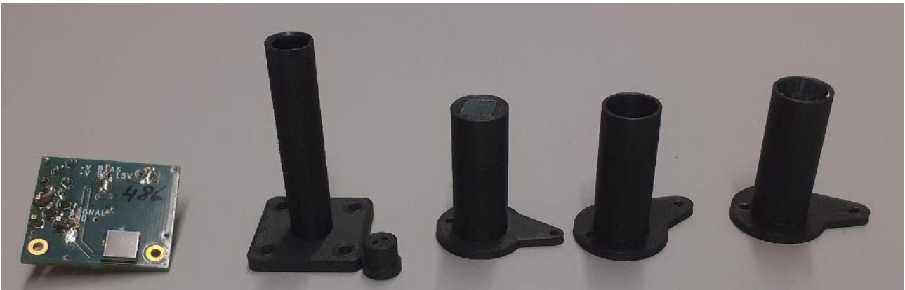
Figure 5.30: From left to right: the SiPM used for the measurement, T1, sT2 (with foil), rT2 (no foil), rT2 (with foil) used for the measurements of the light output of fibres in air.
