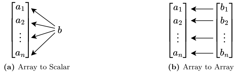
Figure 4.10.: Default calculation mapping when using NumPy arrays without explicit dimension commands. Note that fig. 4.10b only resolves if the dimension of both arrays has the same size.
