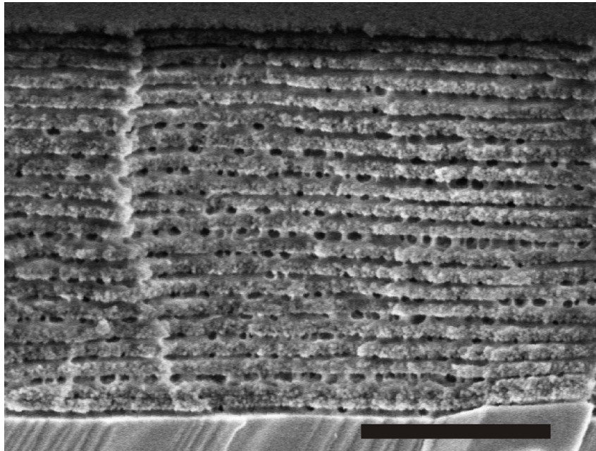
Figure 5-5.: Cross-section SEM image of the spincoated PMMA/SiO 2 -stack. The scalebar equals 1 \mu\text{m} .
