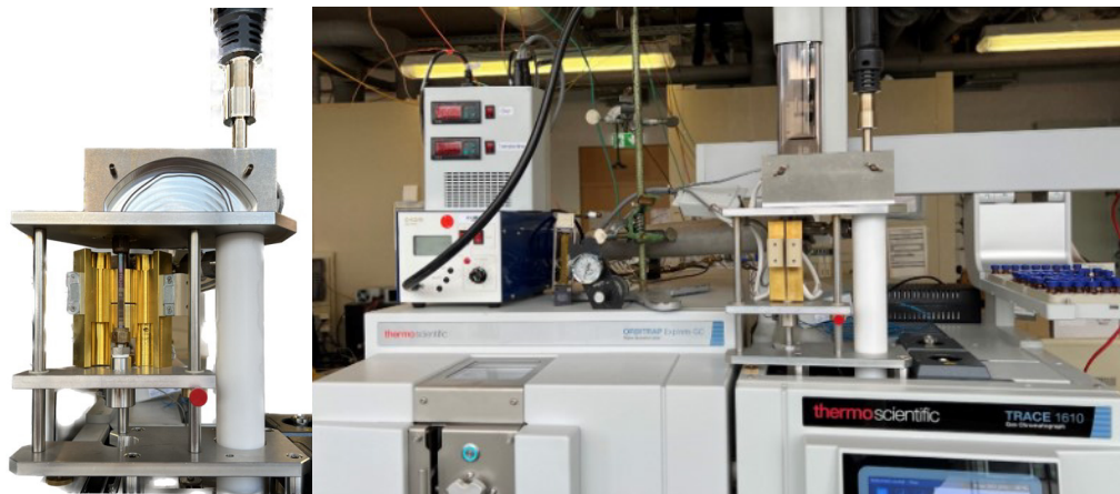
Figure 2.8 The image on the left shows the Versatile TD injector, while the view on the right displays the entire system, including control systems and installation on the GC-MS.
