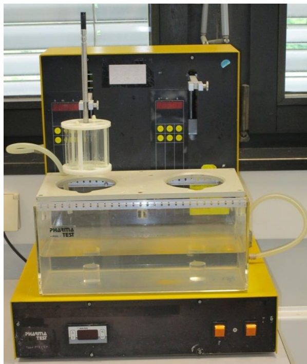
Figure 3: European Pharmacopoeia disintegration apparatus. a) Laboratory setup (PTZ 2 EH, Pharma Test, Hainburg, Germany. b) Schematic representation of the basket-rack assembly (Ph.Eur., European Pharmacopoeia, 2014). Dimensions in mm.
