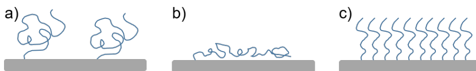
Figure 2.7: Schematic of the possible conformation of surface grafted polymer chains. a) The weak or repulsive polymer-surface interaction results in a polymer coil. The conformation is referred as "mushroom" like structure. b) The strong surface-polymer interaction leads to adsorption of the polymer chain on the surface. The resulting conformation is referred as "pancake" conformation. c) The density of the grafted polymer chain is high. The overlap of the polymer chains results in stretched polymer chains. The resulting conformation is referred as "brush" like structure. [22] The figure was made after Ref. [22,59]
