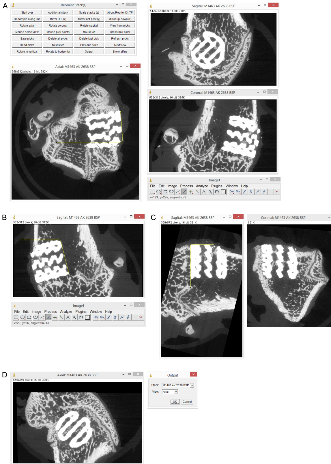
Fig. A.5: Reorientation with the Align Stacks plugin. A - Control unit and individual view from three-dimensional axes, B - Angle measurement with the angle tool, C - Control of alignment, D - Generation of an axial output file.
