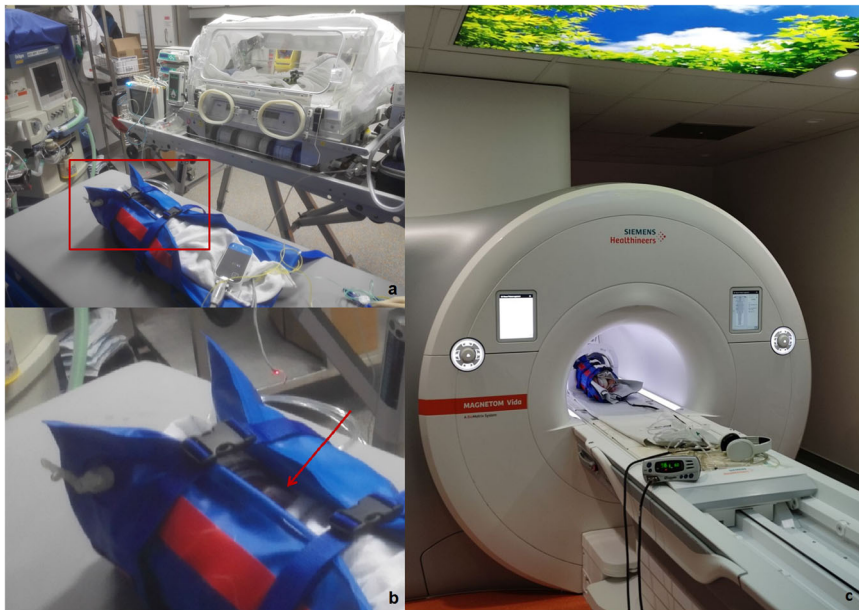
Fig. 1 immobilisation of a premature patient in the MR preparation room. The child is transferred from the incubator into the vacuum mattress, MR-compatible monitoring is applied (a) and a pacifier (b, red arrow) is used. After vacuum has been applied, the child is taken into the MR scanner (c)
