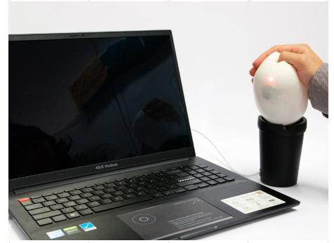
Figure 1: Pressure-gesture-controlled lamp using barometer data, by Olman Arias Valverde.
