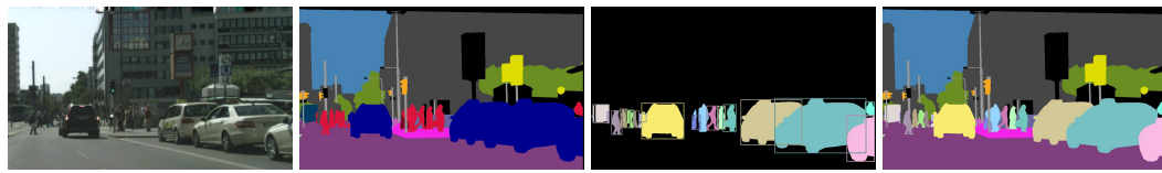
(a) City / traffic scene with several cars, buildings in the background, road and sky. (b) Semantic segmentation of all classes. (c) Instance segmentation with different labels for the same class. (d) The combination of instance and segmentation type forms the panoptic segmentation.
