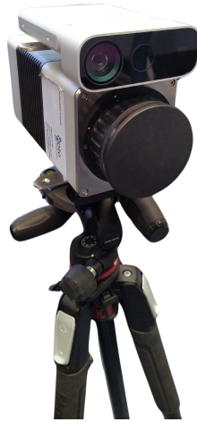
Fig. 4.3.: The stereo hardware setup with Azure Kinect (top) and VarioCam HD (bottom) forms a fixed stereo system mounted on a tripod.
