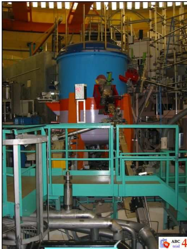
Figure 2.1: The UCN turbine at "niveau" D at the ILL in Grenoble. The vertical neutron guide enters the turbine in the center of the picture[48].
