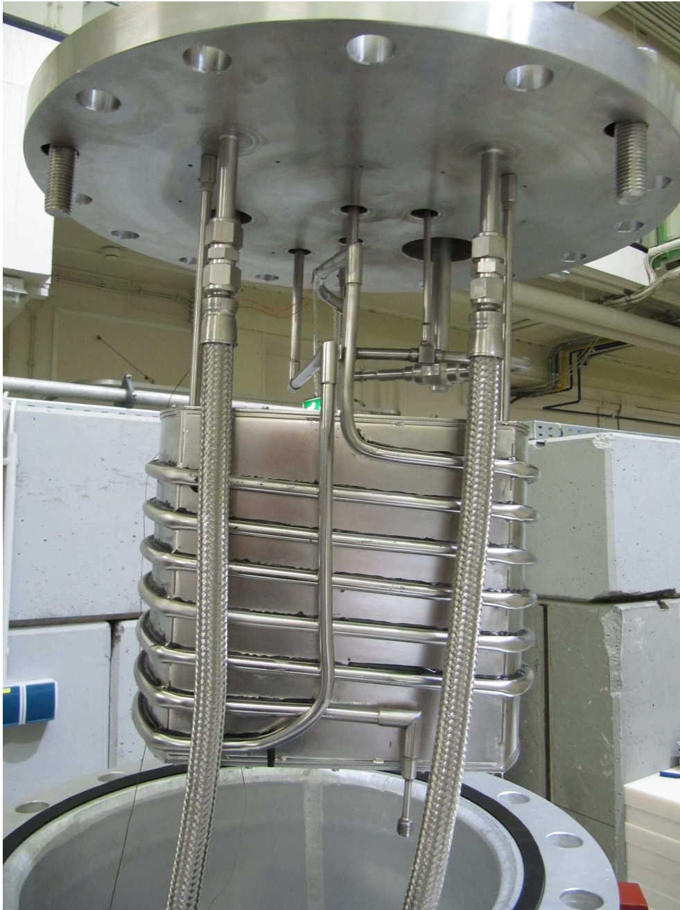
Figure 6.5: Picture of the helium buffer volume which is already connected to the top flange of the support volume outside the reactor. The two swagelok lines in front are the D_2 and premoderator connections to the neutron guide and the premoderator transfer tube.
