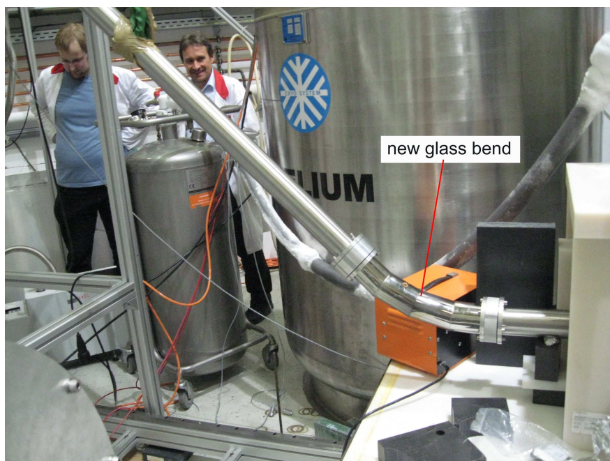
Figure 4.27: Picture of the new 45 degree glass bend coated inside with 500 nm NiMo(see chap.7.5) installed at the UCN source yield.
