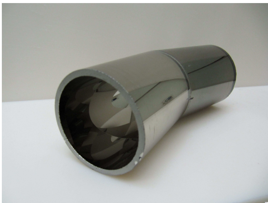
Figure 7.29: First self made glass bent coated in the new sputter facility in Mainz.
