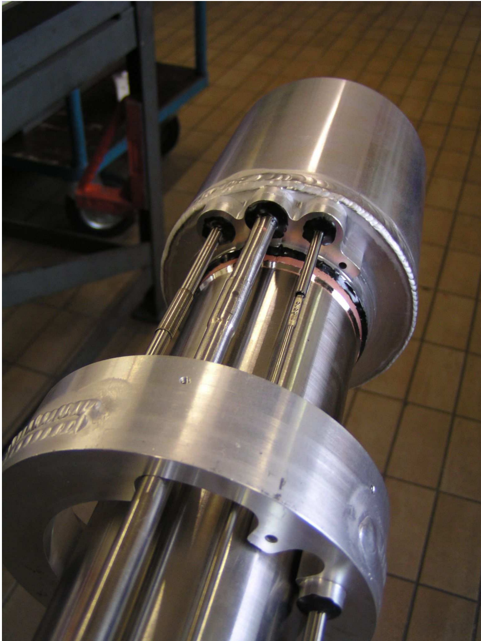
Figure 6.6: Picture of the nose during the final soldering of the cryogenic transfer lines. The 70 mm aluminium stainless steel transition can be recognized on the glossy copper coating. All the other transitions are hidden by low temperature stycast (black), in order to avoid oxidation of the copper in air.
