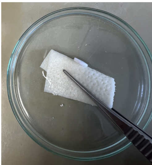
Figure 2 Hybrid material of hAD with printed PLA-structure after a 72-hour incubation in PBS. hAD, human acellular dermis; PBS, phosphate buffered saline; PLA, polylactide.
