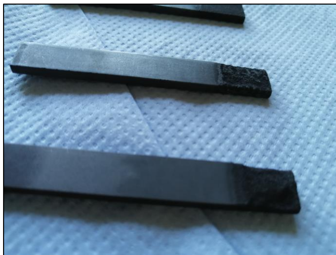
Figure 22. Heavy corrosion of graphite cathodes when LiBr was used.
