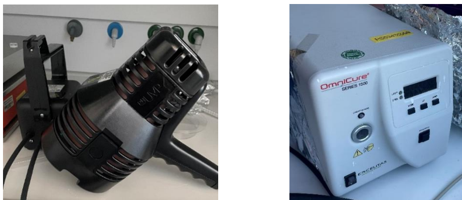
Figure 3.2: On the left side the Black-Ray B-100 AP High Intensity UV lamp from UVP used in the original microfluidic setup. On the right the OmniCure series 1500 from Excelitas which replaced the left lamp in the improved microfluidic setup.
