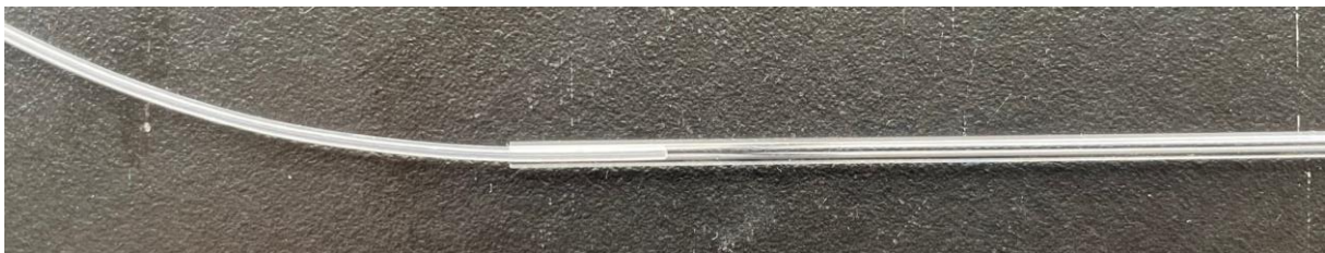
Figure 3.6: Glass capillary to be integrated into the microfluidic experimental setup. Its inner diameter is large enough to insert the polyethylene tubing, however the connection point has to be sealed.
