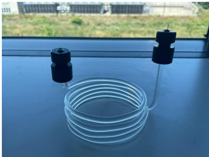
Figure 3.4: Glass spiral with its needle connection on both ends. The radiation source can be placed in the center to evenly irradiated the circling droplets.
