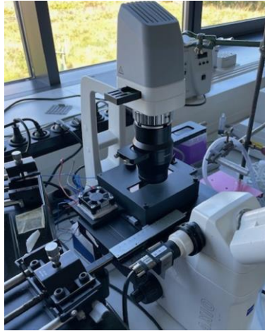
Figure 7.8: Closed irradiation chamber underneath the microscope allowing the creation of core-shell particles with negligible connection between the two.
