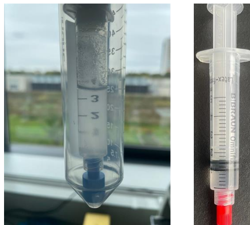
Figure 7.4: Syringe stopper in place on the left allowing centrifugation of the core-particle dispersion within the syringe. After centrifugation the excess water is removed and the syringe piston carefully inserted resulting in the core-particle paste ready for use in core-shell microfluidics as shown on the right.
