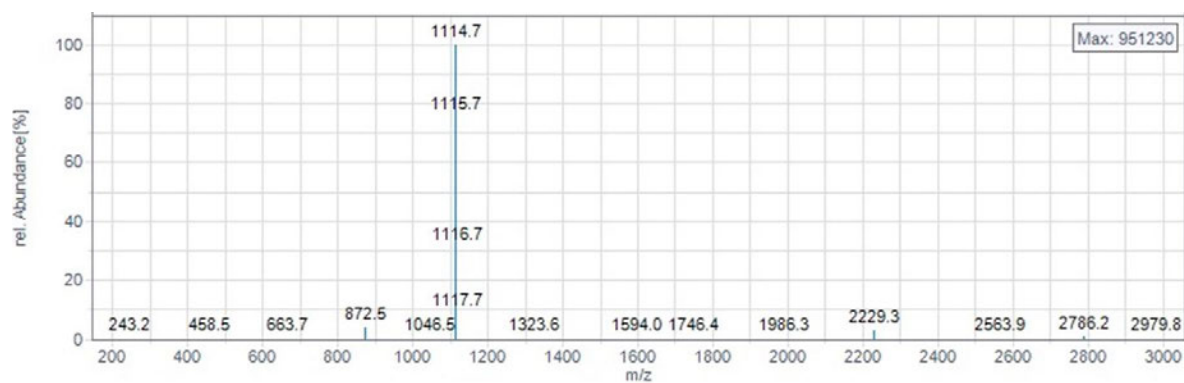
Figure 10.24: Mass spectrum (LC-MS, Method F, figure 4.9) of Synthesis of H-L-Lys(pentynoyl)-D-His(Trt)-L-Trp(Boc)-OH.
