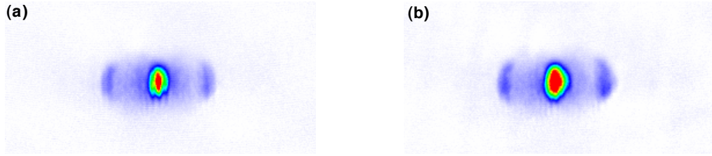
Figure 6.10: (a) presents the absorption image of an 1D lattice that was illuminated by the electron beam, while (b) shows the corresponding image without electron beam exposure.
