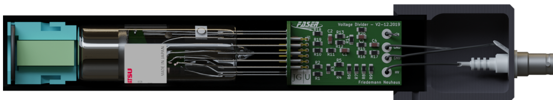
Figure 10.5: Rendering of the readout assembly for the calorimeter. The tube and the end-plug are cut open to allow visibility of all components. The components from left to right are: the filter holder (light blue) with both the filter (black) and the light mixer (light green), the photomultiplier connected to the voltage divider via the adapter PCB and the end-plug with the electrical connections.
