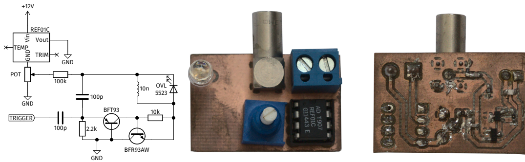
Figure 11.4: Schematic for the first prototype of a LED driver with adjustable bias voltage and the fabricated board.
