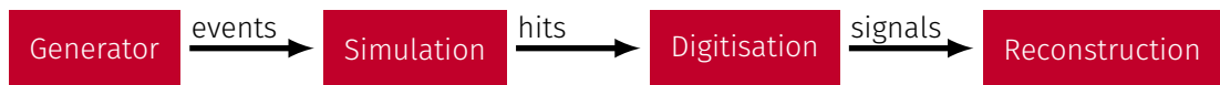
Figure 5.5: Simplified flow diagram of the ATLAS event simulation chain with the algorithms drawn in boxes and the objects created written over the arrows.
