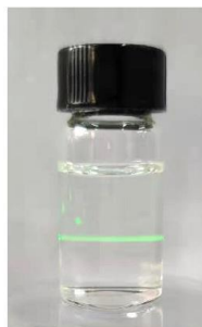
Figure S5. Photograph of the Tyndall effect observed for the colloidal suspension of Ce-POM in acetonitrile after storage for one year.
