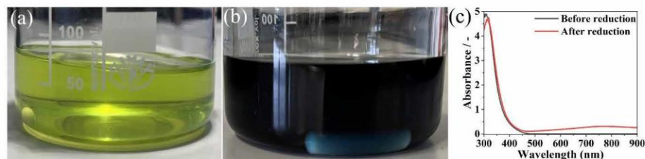
Figure S1. The optical photographs of PMo 12 in DMF solution before (a) and after (b) reduction, and corresponding UV-visible spectra after being diluted to 1/10 of original concentration.
