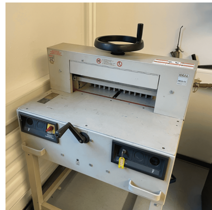
(d) Paper cutting machine for PE foil preparation.
