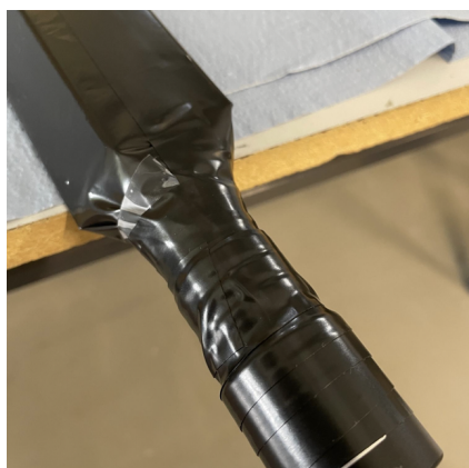
(c) Transition from PMT to high-voltage socket fully wrapped.
