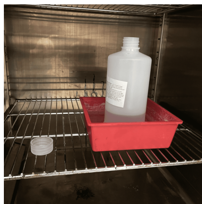
(b) Component A inside oven for decrystallization.
