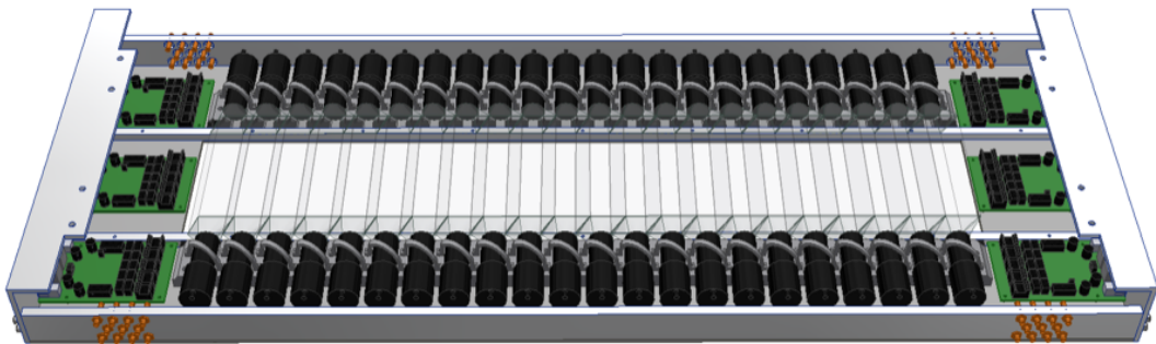
(b) 22 trigger detectors and six DAC boards are held by the trigger layer mounting.
