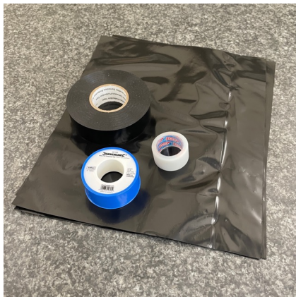
(c) PTFE tape, sealing tape, tesafilm invisible®, and PE foil cut.
