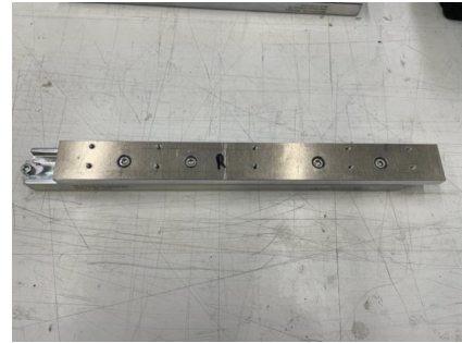
(b) Screw right adapter profile to telescopic rail.
