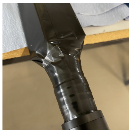
(b) PMT covered with sealing tape.
