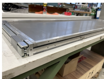
(d) Mount front profiles as required.
