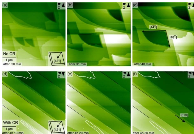
Figure 2.7: AFM image series of calcite (104) surface under time lapse without additive (a-c) and with Kongo red as additive (d-f). (a-c) Show classical etch pit formation over time while Kongo red terminates the polar step edges and inhibits dissolution of \text{CaCO}_3 for growth of etch pits from a supersaturated solution. The figure is reprinted with permission from Langmuir. [6]
