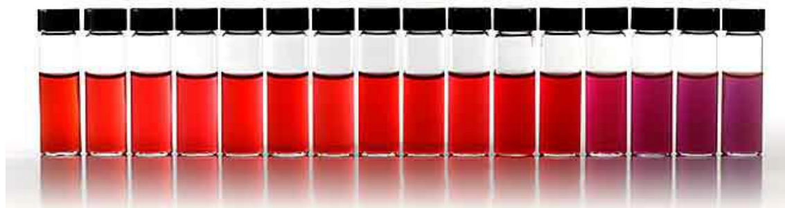
Figure 2.25: Plasmon absorption shift of Au nanoparticles f.l.t.r. up to 20 nm diameter. Image Source: Sigma Aldrich Webpage February 2015.
