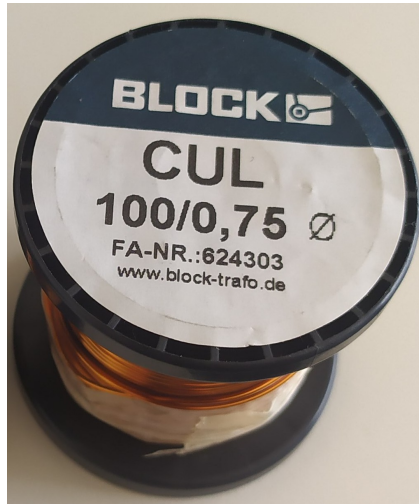
Figure 4.7: Photo of enameled copper wire used in the Goubau line test stand.
