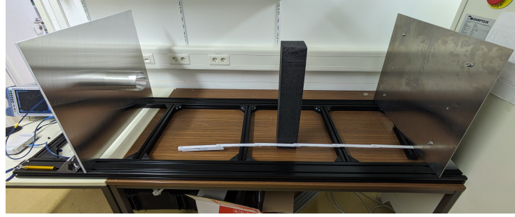
Figure 7.1: Photo of wire test stand with hard foam block.
