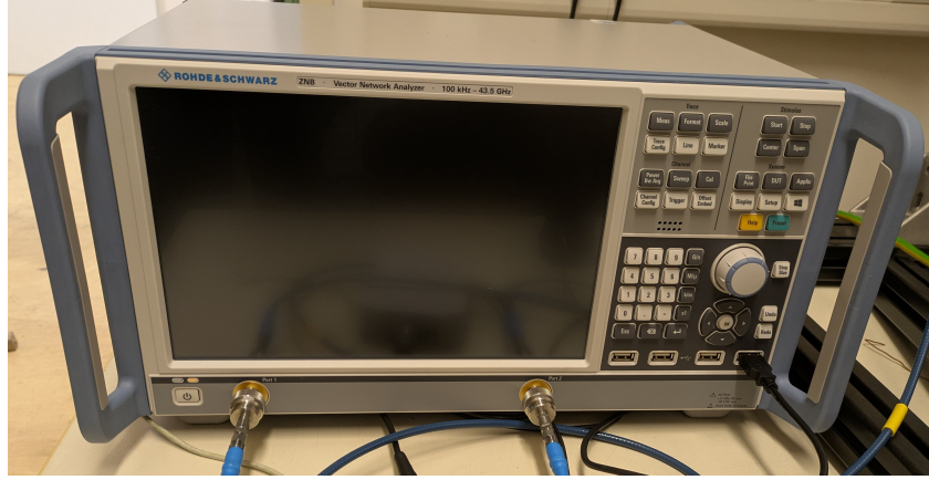
Figure 4.5: Photo of the Rohde und Schwarz ZNB vector network analyzer used for the Goubau line test stand.
