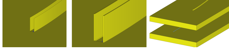
Figure 7.14: Different model representations of shielding foils. Sheet representation on the left, modeled foil thickness of 0.1 mm in the middle, and a 3 mm solid block with carved slit on the right.
