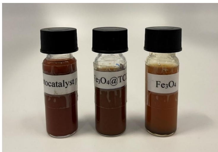
Figure 59. Image of magnetite dispersions before and after the modifications: pristine magnetite nanoparticle dispersion in DIW (right), magnetite nanoparticles modified with TCDS \text{Fe}_3\text{O}_4@TCDS (middle), and magnetite nanoparticles encapsulated with photocatalytic polymers (left).
