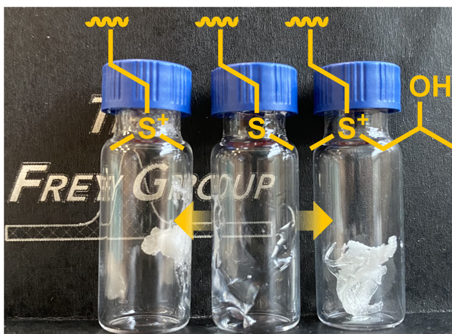
Figure S29: Visualization of the changed properties of the copolymer (middle) after the functionalization through alkylation with methyl iodide (left) and alkoxylation with propylene oxide (right).
