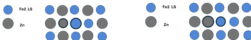
Figure S62: Optimisation of the Model 1 (left) to Model 2 (right). Note that considering the size of the optimised molecules Model 2 represents the double-site defect in the lattice. For the further calculations the Zn molecule in position 2 must be changed to the HS-Fe1 one. The corresponding Model 3 is shown in Figure S60 . The molecules that are subsequently optimised are marked with the thicker rim.
